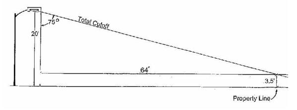
Figure D: Luminaires With No Cutoff or a Cutoff Angle Greater than 75 Degrees
