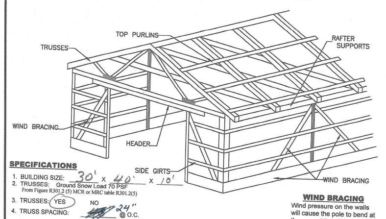
the ground line. A WIND BRACE should be provided at the eave line for buildings with a side wall height of over 10', and for buildings 60' long and over. The BRACE should be a 2" x 4" at lease 12' long, extending from the pole to the rafter at an angle of 45 deg to the
