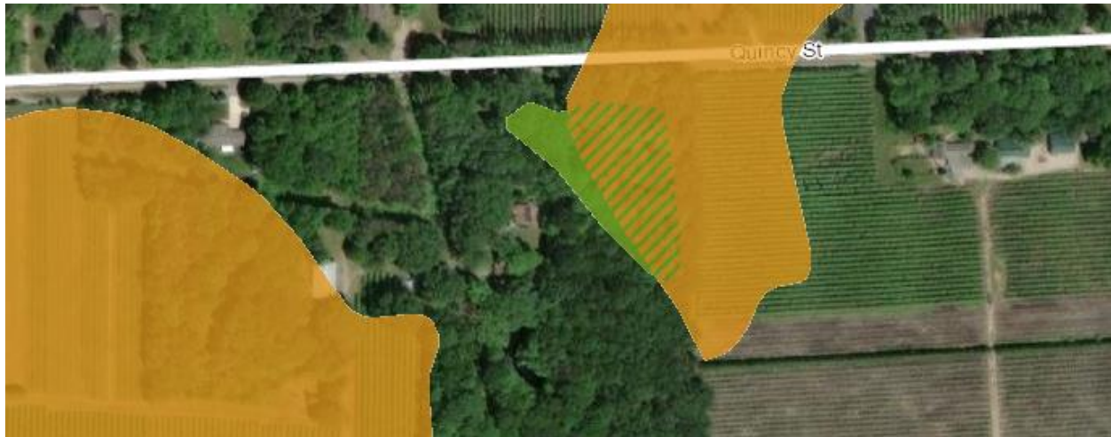
Figure 5. EGLE wetlands map. Wetlands are shown in green, wetland soils are shown in orange, and when both are present they are shown in striped green and orange.
