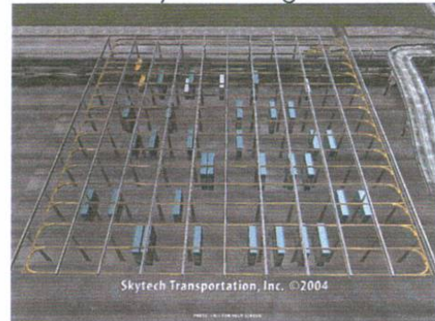
A typical SkyTech Transportation GRID layout set next to a rail line for train assembly. The GRID allows for optimization of storage capacity and enhances land usage.
