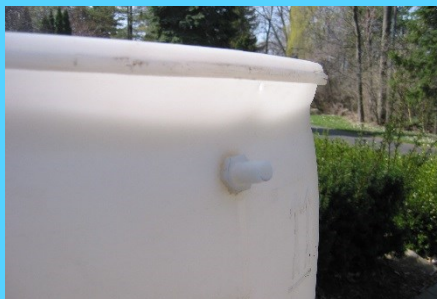
Upper hose barb for water overflow.
